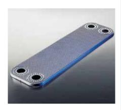
By allowing water to flow more evenly, the Micro Plates<sup>™</sup> make better use of their surface area to generate maximum turbulence to improve overall system efficiency. Between the fastest and slowest flowing areas, the difference is only x 3, as opposed to x 10 in older heat exchanger models, which distributes and mixes fluid better to maximise heat transfer.
