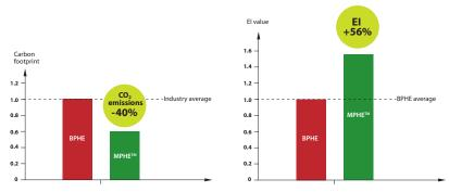
Our MPHEs improve the flow across the plate and utilisation of the surface area for better heat transfer. Compared with traditional brazed plate heat exchangers, MPHEs have an Exchanger Index (EI) value up to 56% higher under the same working conditions.
