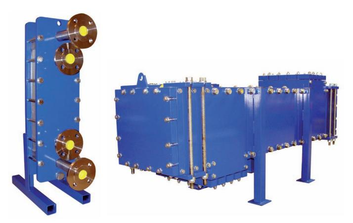
The **SAW** heat exchanger is built into a frame with its welded plate pack. The perfect solution for heat transmission duties, which cannot be handled in a normal gasketed plate heat exchanger because of a too high design temperature, design pressure, or if there is no suitable gasket material for the media which are to be treated in the heat exchanger.
