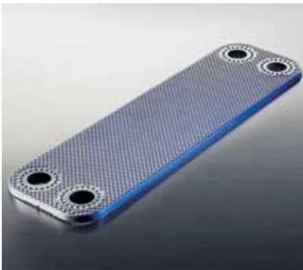
By allowing water to flow more evenly, the Micro Plates™ make better use of their surface area to generate maximum turbulence to improve overall system efficiency. Between the fastest and slowest flowing areas, the difference is only x 3, as opposed to x 10 in older heat exchanger models, which distributes and mixes fluid better to maximise heat transfer.
